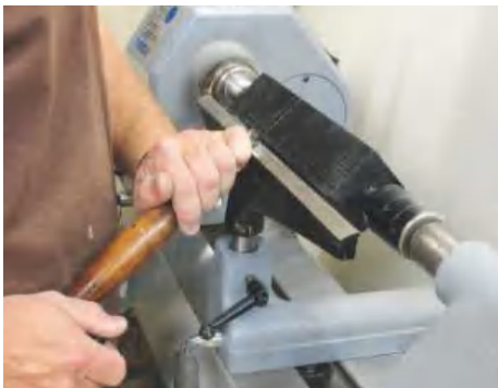
▲ Pic.7 The stance used is normal for most of the tools. The left hand is generally over the tool, which creates a tunnel for the tool to be rotated in
